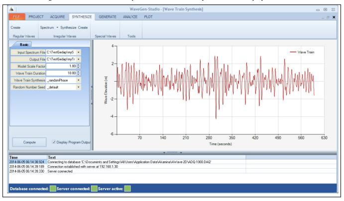
The system uses a network of connected servers to provide the necessary data acquisition and control capabilities. Data acquisition servers allow data to be acquired from sensors used in the study and control servers are used to control the electric or hydraulic actuators to generate waves.
