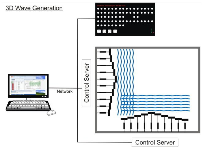
Figure 3: 3D Wave Generation with Operator's Interface, Data Acquisition Server and Control Servers
